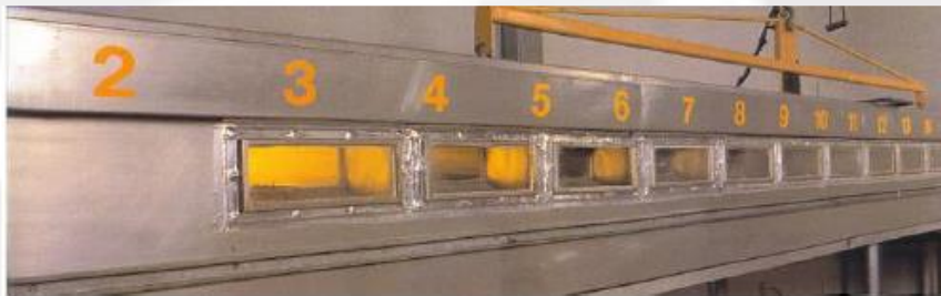
Steiner Tunnel used to test cable per UL 2024
